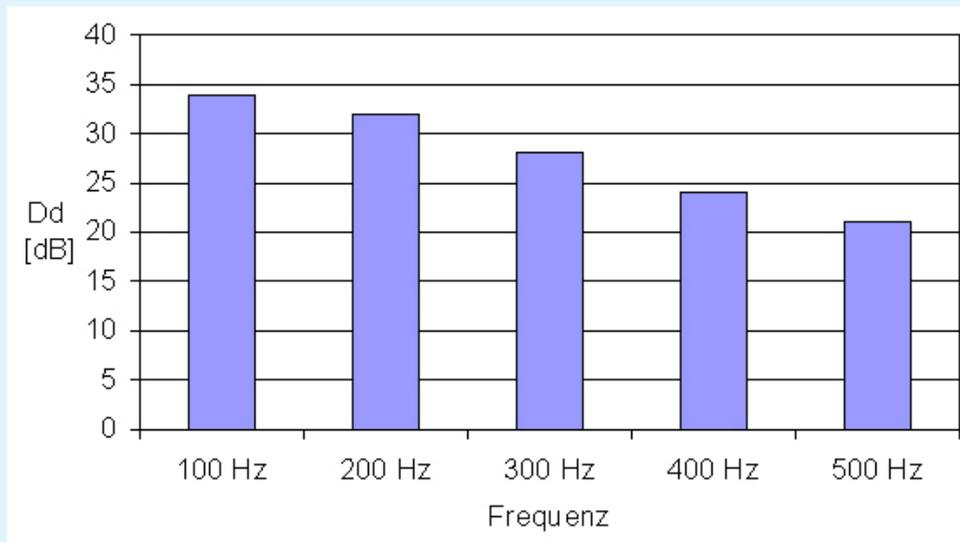
Measured transmission loss of the new reflection silencer
