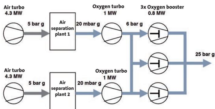
Fig. 2: Compression process schematic (from 1962)
