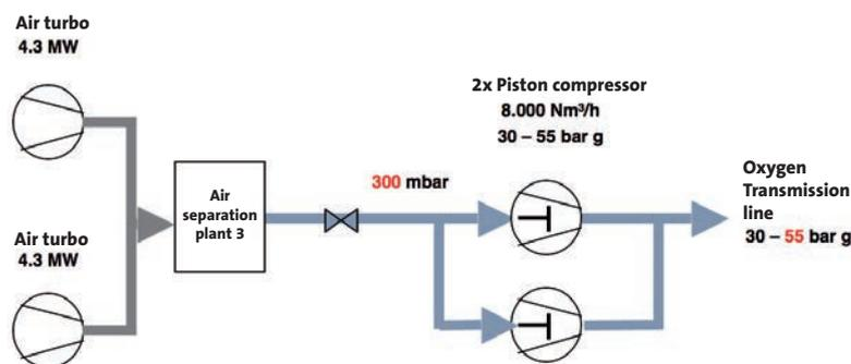
Fig. 5: Process schematic for new O<sub>2</sub> compression concept (from 2014)
