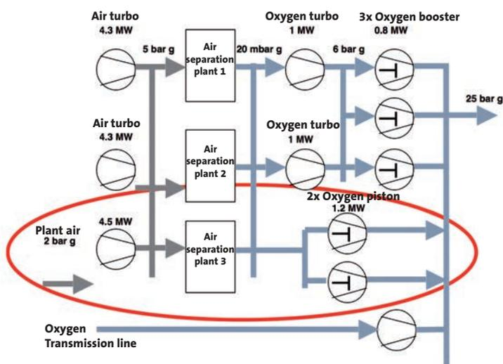
Fig. 3: Compression process schematic (from 1989)
