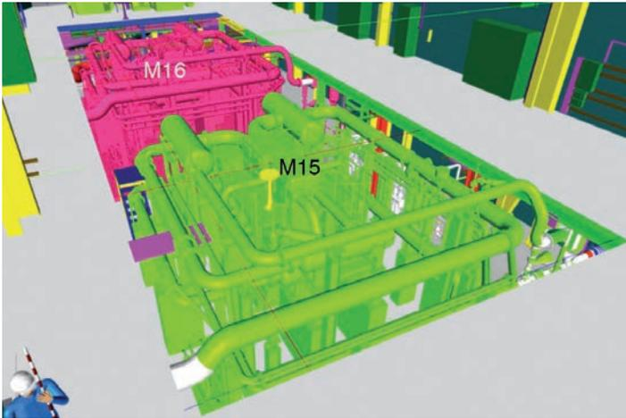
Fig. 7: Interior view of the hall (CAD model) from above onto the two new oxygen piston compressors M15 and M16 with the foundations in the basement, shown without the concrete walls (safety barriers) around the compressors.
