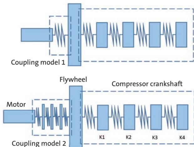
Fig. 9: Schematic layout of the drive train model for the torsional analysis. Top: simplified connection, bottom: extended coupling connection.
