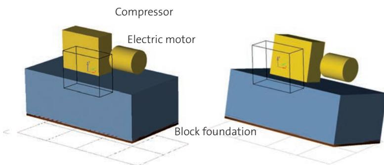
Fig. 12: Two chosen examples of the 6 possible basic eigenmodes of the machine installation (schematic) on the elastic floor. Lattice model of the compressor and the lower level of the block foundation: non deflected position, left: eigenmode with vertical deflection only (lift eigenmode), right: tilting around the longitudinal axis (rocking mode).
