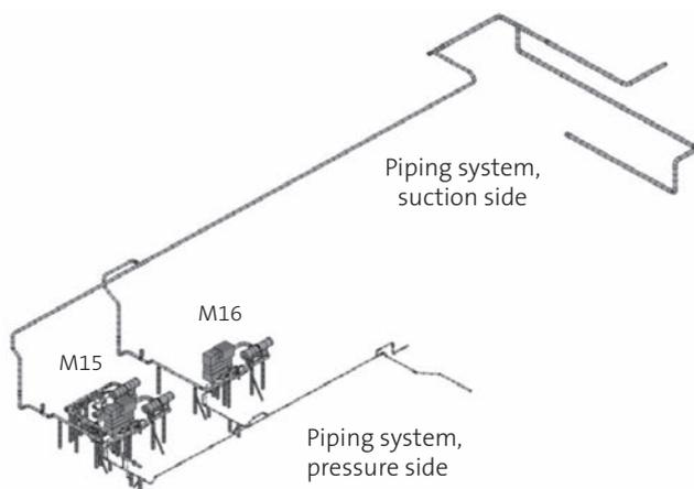
Fig. 8: Sketch of the piping system model space for the pulsation and vibration analysis (source: Burckhardt Compression AG).
