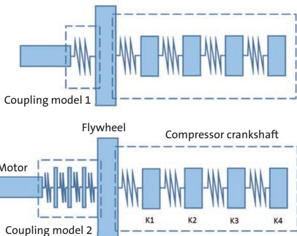
Fig. 9: Schematic layout of the drive train model for the torsional analysis. Top: simplified connection, bottom: extended coupling connection.
