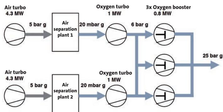
Fig. 2: Compression process schematic (from 1962)
