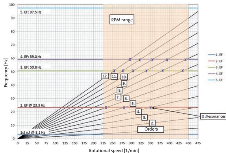
Fig. 11: Resonance diagram (Campbell diagram) for the torsional resonance frequencies of the oxygen compressor up to the 5th eigenmode (EF) and 12th order of the rotational speed, red field: operating speed range of the compressor.
