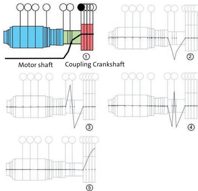
Fig. 10: Calculated torsion eigenmodes (heavy line) - no. 1 (3.1 Hz), no. 2 (23.3 Hz), no. 3 (50.8 Hz), no. 4 (59.0 Hz), bottom: no. 5 (97.5 Hz).
