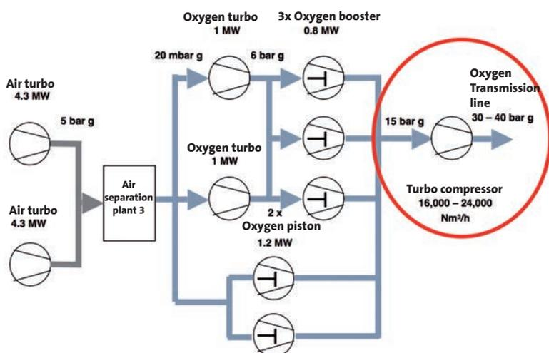
Fig. 4: Compression process schematic (from 1998-2015)
