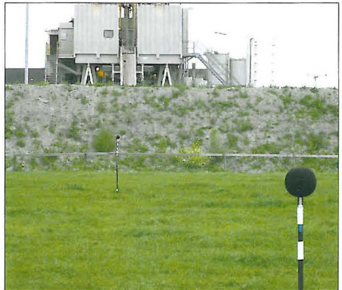
Fig. 5 Drilling rig with noise measurement equipment
