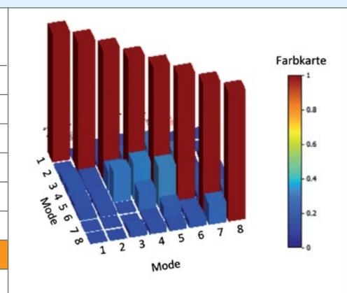
Natural frequencies of the plant and 3D illustration of the MAC matrix at the example of the CFDD results
