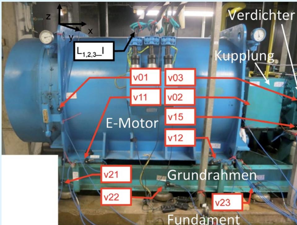
Drive of the coolant compressor plant with vibration and current measuring points
