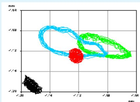
Orbit display of shaft vibrations of the turbines (black and red) and pinion shaft (blue and green) at part-load – 2 MW
