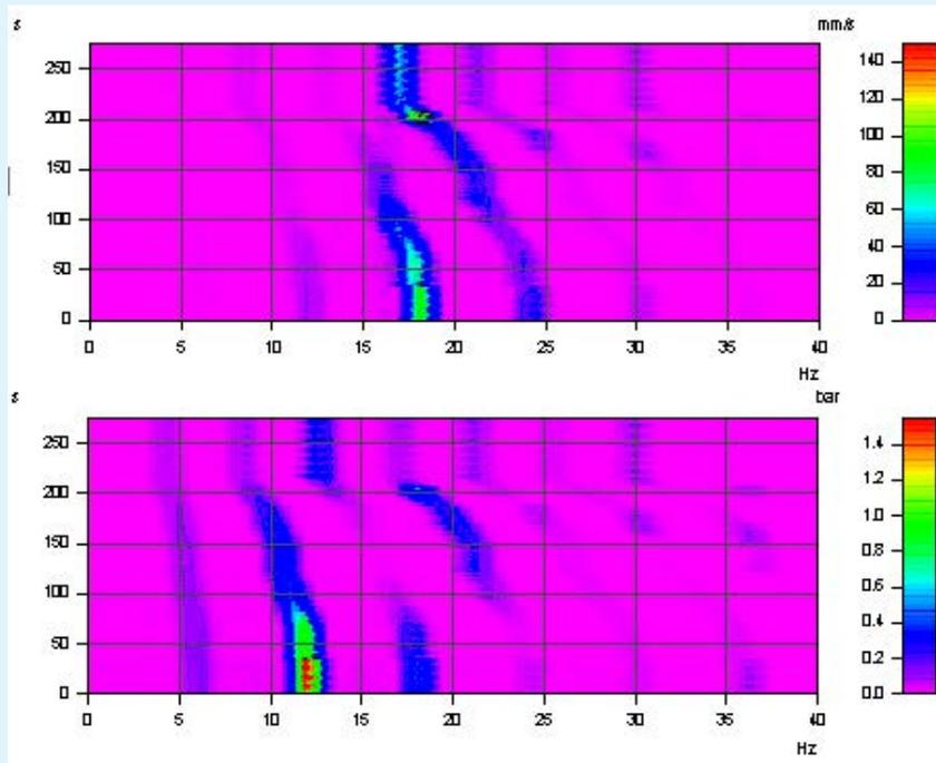
Time-frequency-amplitude spectrum at shutdown of compressor rotation speed from 374 1/min to 262 1/min, top: structural vibrations at the interstage of the pipe with local resonance at approx. 18 Hz, bottom: pulsations at the interstage pipeline
