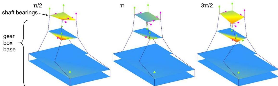
**Figure 3.** Wire frame model and EFDD mode shape freeze images of the refrigeration system at 2,158 Hz.
