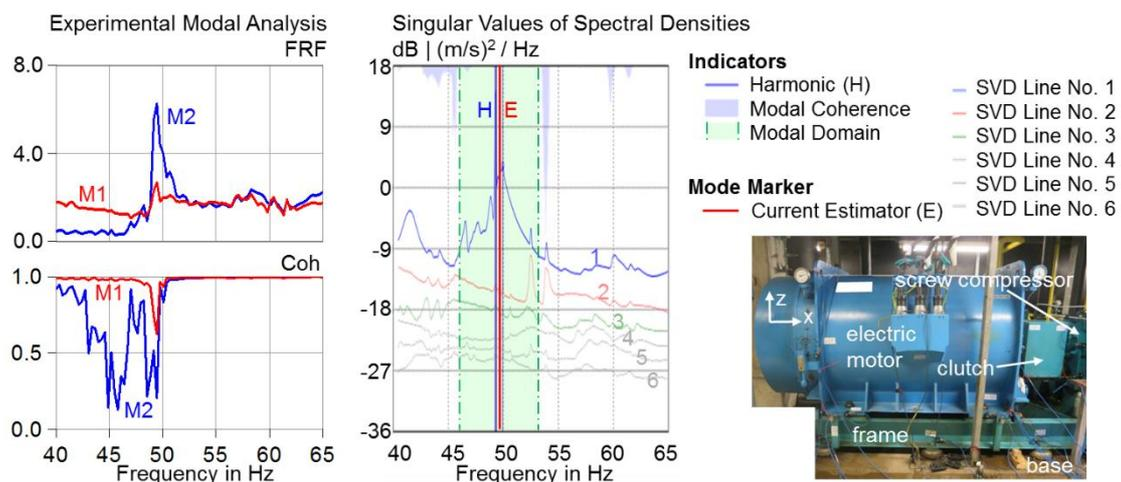
**Figure 1.** Left: Details of Frequency Response Function (FRF) with peak and Coherence (Coh) with collapse at 49.9 Hz. Center: Corresponding details of SVD data for OMA. Right: Photo of the compressor package.
