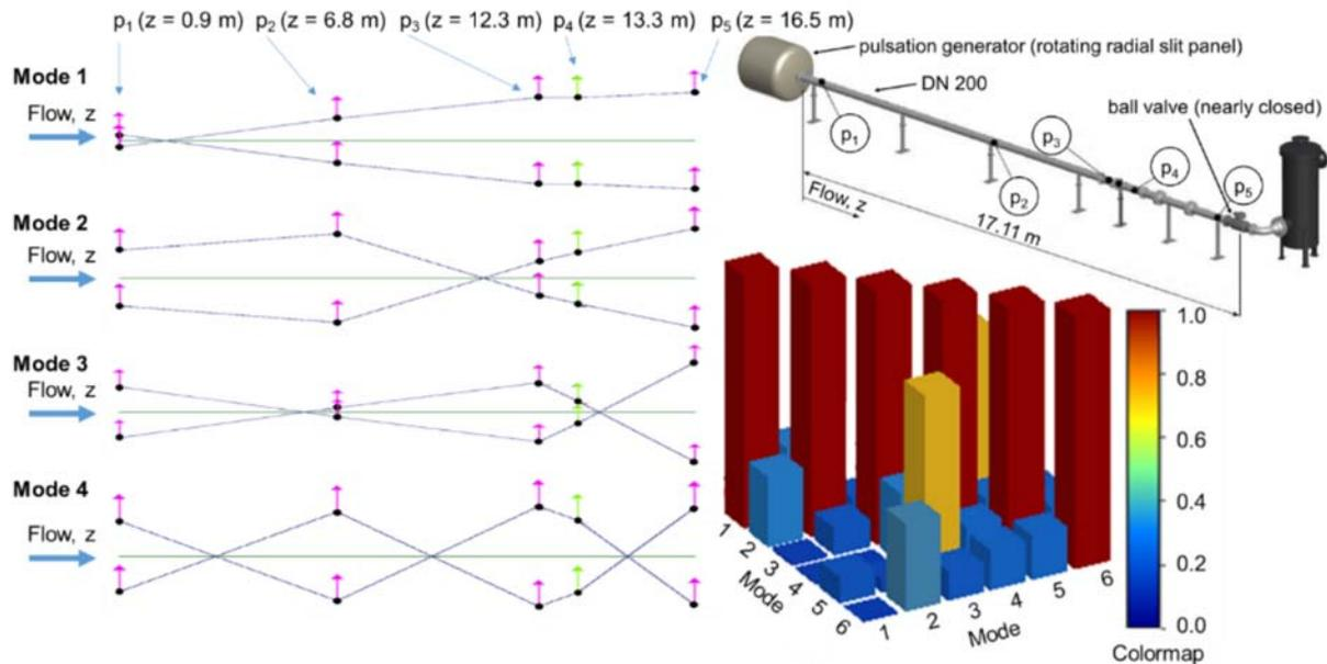
**Figure 4.** Left: First four pulsation mode shapes of the test section without spatial aliasing. Right: Drawing of test section (top) and MAC-matrix (bottom).
