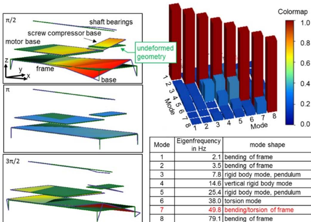
**Figure 2.** Left: Wire frame model and CFDD mode shape freeze images of the refrigeration system at 49.9 Hz. Right: CFDD MAC-matrix (top) and mode list (bottom).
