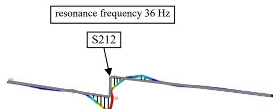
**Figure 10:** Calculated mode shape of the piping at the resonance frequency of 36 Hz in the area of measuring point S212.
