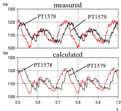
**Figure 6:** Measured and calculated pressure pulsations at the interstage of compressor A (original situation).
