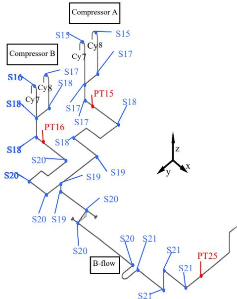
**Figure 3:** Sketch of the discharge piping, 2<sup>nd</sup> stage, (B-flow) of both compressors and the pipe vibrations (e.g. S170) and pressure pulsations (e.g. PT1604) measuring points.
