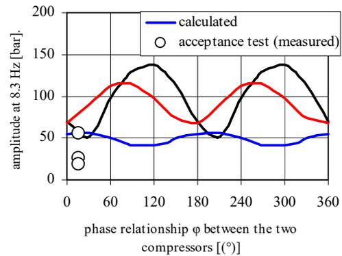
**Figure 8:** Pressure pulsation amplitudes of the B-flow for the frequency of 8.3 Hz in the planned situation with increased mean static discharge pressure versus the phase relationship  $\varphi$  between the two compressors.
