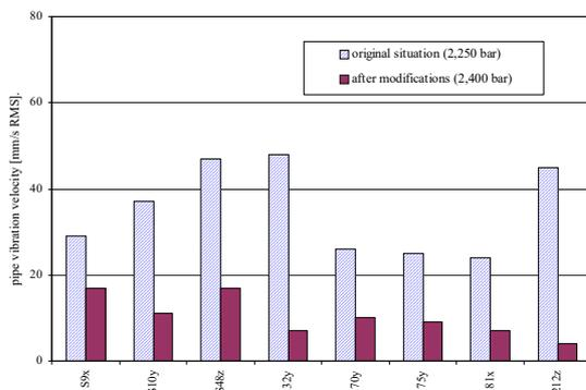
**Figure 11** Measured pipe vibrations in the original situation and after realisation of measures for the increased discharge pressure of 2,400 bar.
