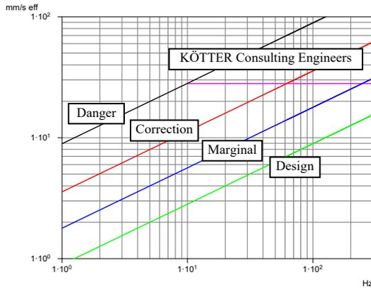
**Figure 1:** Orientation values of allowable piping vibrations with a stationary flexural stress and strain.
