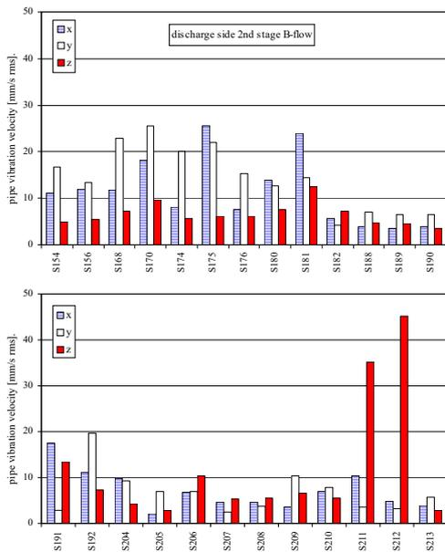
**Figure 5:** RMS vibration velocities (2 - 1,000 Hz) of the piping of the B-flow on the discharge side, 2<sup>nd</sup> stage.
