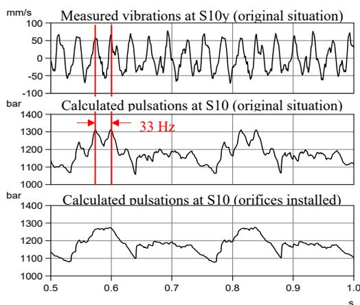
**Figure 9:** Measured pipe vibrations at the measuring point S10 (top) and calculated pressure pulsations (centre) in the original situation as well as calculated pressure pulsations (bottom) with installed orifices.
