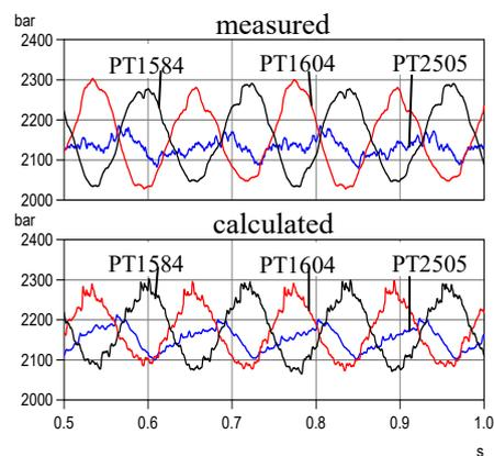
**Figure 7:** Measured and calculated pressure pulsations at the discharge side of the 2<sup>nd</sup> stage B-flow (original situation).
