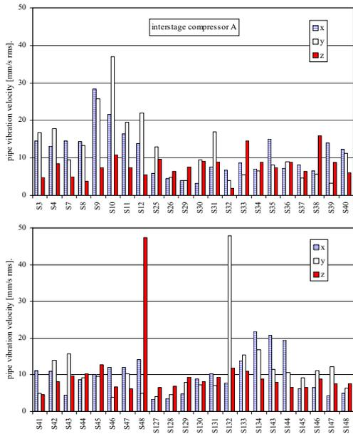
**Figure 4:** RMS vibration velocities (2 - 1,000 Hz) of the piping on the interstage of the compressor A.
