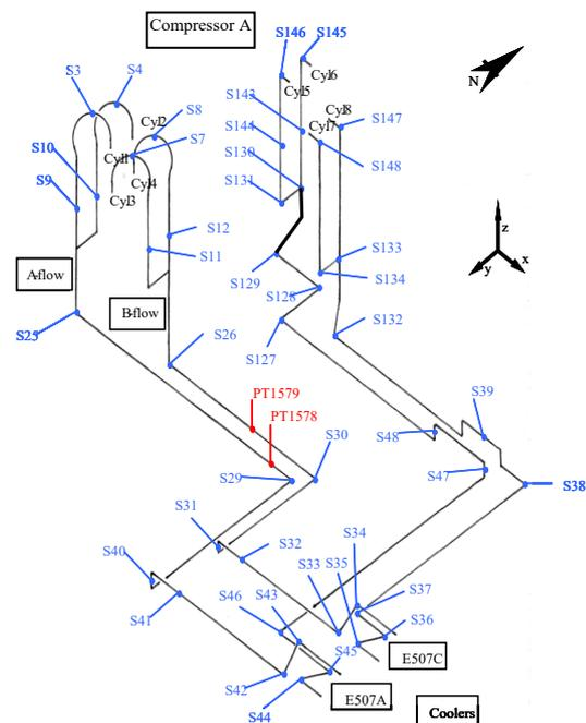
**Figure 2:** Sketch of the interstage of compressor A (A- and B-flow) and the pipe vibration (e.g. S48) and pressure pulsation (e.g. PT1578) measuring points.
