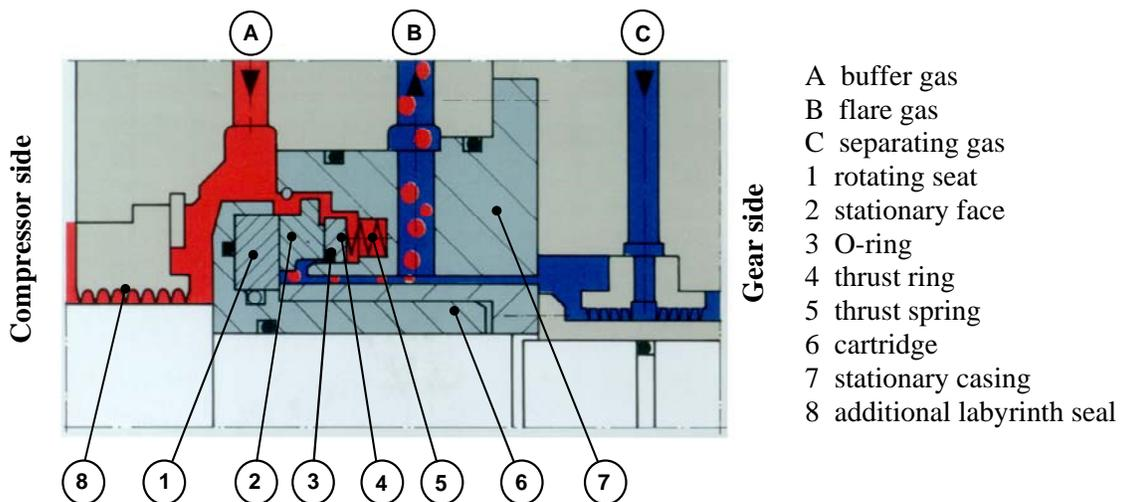
**Figure 2:** Functional arrangement of a dry gas face seal for compressors [1, 2].
