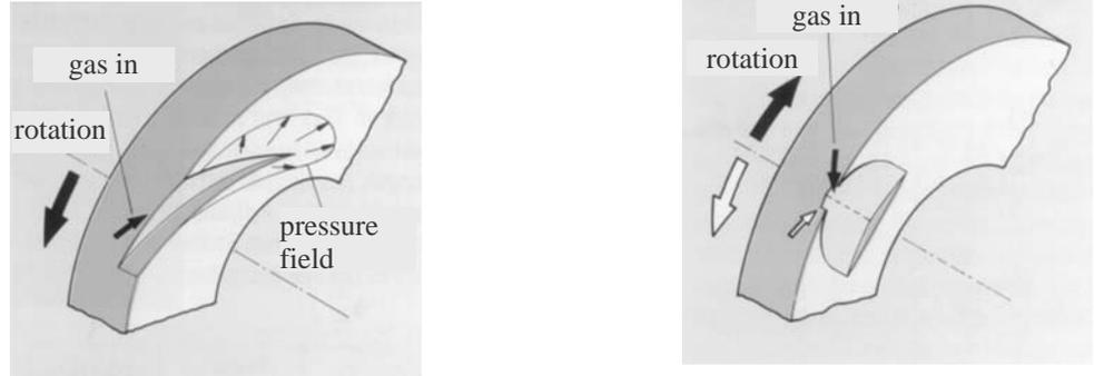
**Figure 3:** Groove geometry, V-groove dependent on direction of rotation (left) and U-groove independent of direction of rotation (right) of the rotating seat [1, 2].
