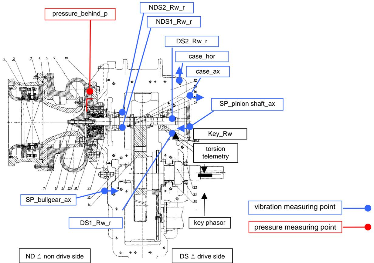
Figure 4: Measuring points at the turbo compressor.
