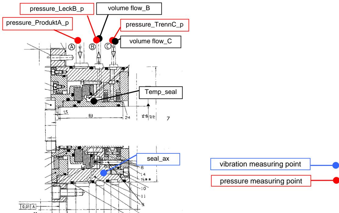
Figure 5: Measuring points in the direct zone of the seal.
