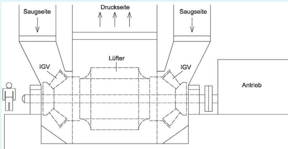
Principal draft of the double-barrelled radial fan with suction and pressure ducts.
