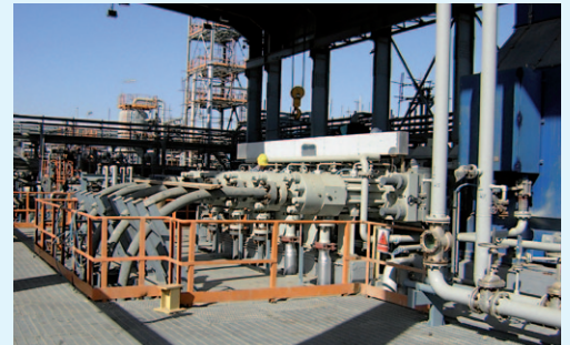
The core of LDPE production: the hyper compressor
